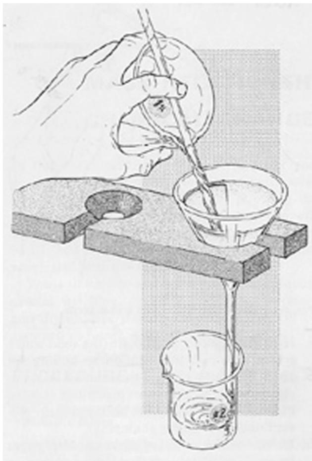
i. Place **beaker #2** under the funnel. The tip of the funnel should touch the beaker so a steady stream can run down the side. Decant the clear liquid from **beaker #1** into the funnel, pouring it into the funnel along a glass rod. A small amount of the precipitate may transfer to the filter paper, but try to keep most of it in the beaker where it can be washed more readily.
