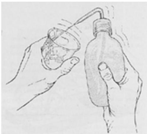
Add the rinse water to the mixture in **beaker #1**. Rinse **beaker #2** again with distilled water and this time discard the rinse water. The clean beaker will be used again in step i.
